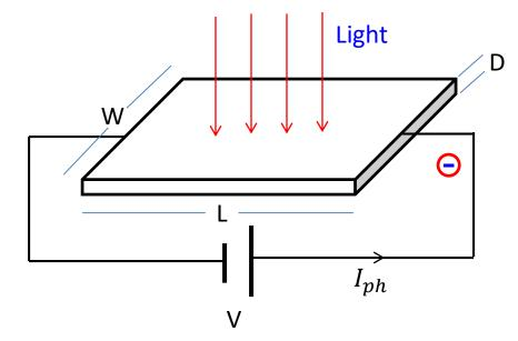
• Assuming unity internal quantum efficiency, then each of these absorbed photons will generate an electron-hole pair(EHP) per sec. If  $G_{ph}$  is the photogeneration rate of EHP per unit volume then
