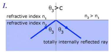
Acceptance angle is the maximum angle  $\theta_{imax}$  which gives just total internal reflection at the core gladding interface
