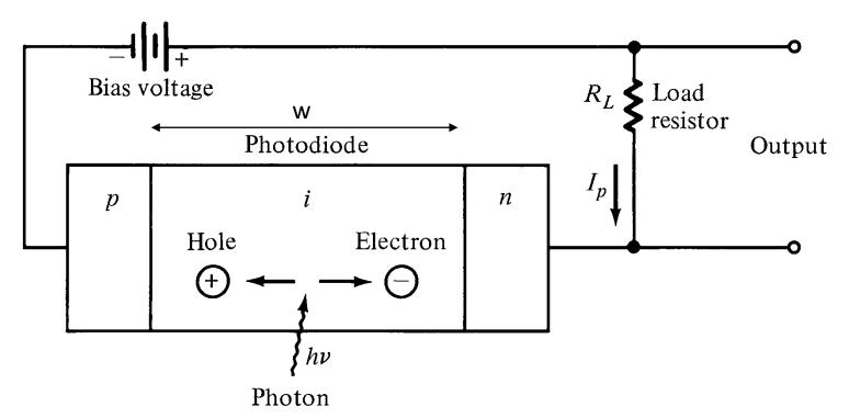
The high electric field present in the depletion region causes photo-generated carriers to Separate and be collected across the reverse –biased junction. This give rise to a current Flow in an external circuit, known as **photocurrent**.
